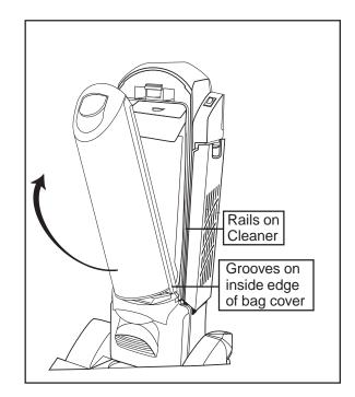
Check the pre-motor filter each time the dust bag is changed. Clean or replace as needed.
